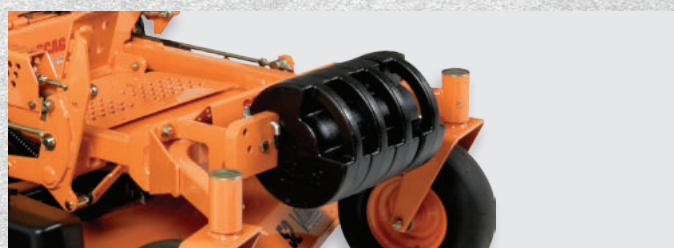
CLAM-SHELL GRASS CATCHER & FABRIC 3-BAG GRASS CATCHER: Both of the catchers include front weights and a mounting bar, keeping the center of gravity low and stable (number of weights depends on catcher and mower model).
