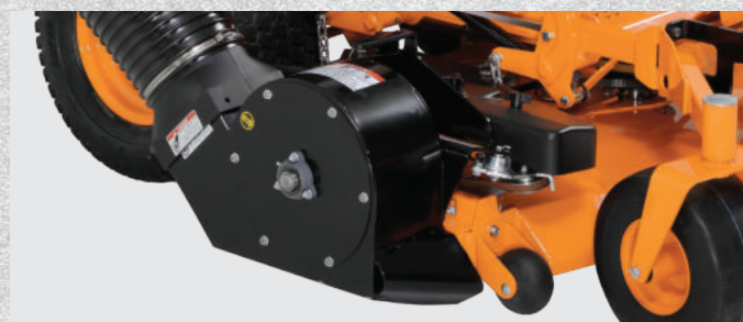
CLAM-SHELL GRASS CATCHER & FABRIC 3-BAG GRASS CATCHER: All spindle-driven catchers have a balanced, all-steel, 4-blade blower that pulverizes debris, reducing particle size to increase packing density.
