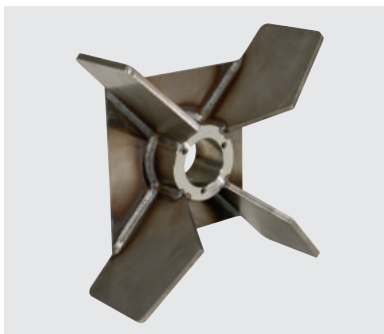
All Scag blower and truck loader impellers are fabricated in-house, then dynamically balanced to ensure ultra-smooth performance and long service life.
