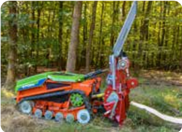
agria 9700e in use with flail mower and optional trailer hitch
